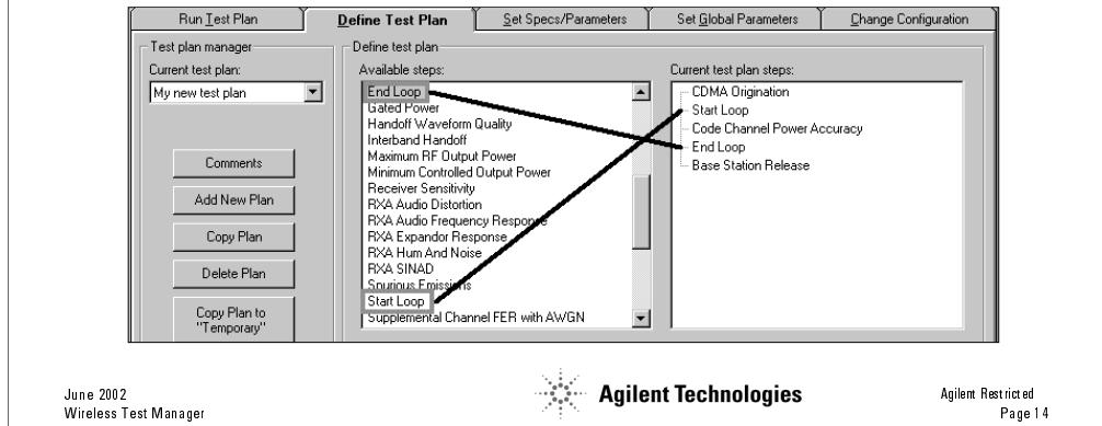
The Start Loop test plan step specifies the start of a looping structure in the test plan. It is one half of the matched pair 'Start Loop' and End Loop which define the start and end of a looping structure.
