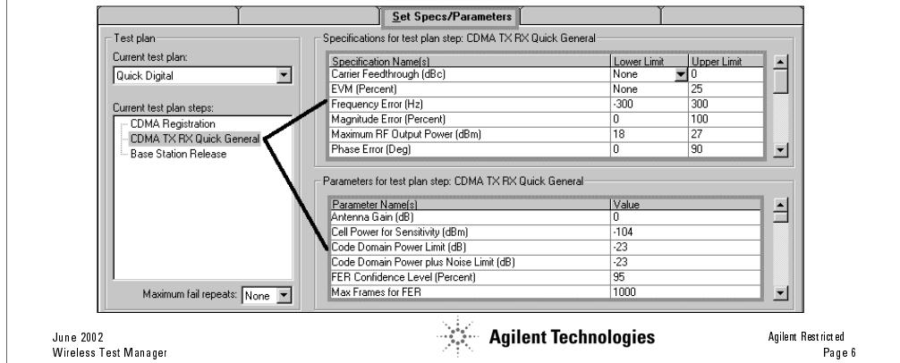
The majority of steps which make up a test plan have their own parameters which you can set to different values. (For example, a step which performs a measurement function may contain a Measurement Timeout parameter.) Any changes you make to parameter values only affects the currently selected test plan.
