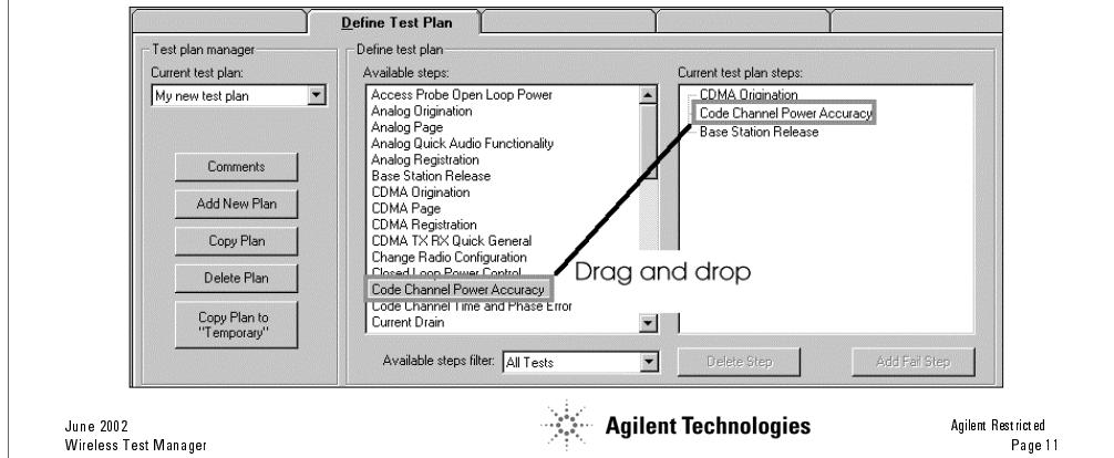
The Wireless Test Manager allows you to add as many steps as you want to your test plan. Test plan steps are run in the test plan in the same order in which they are listed in the Current test plan steps: box on the Define Test Plan tab.
