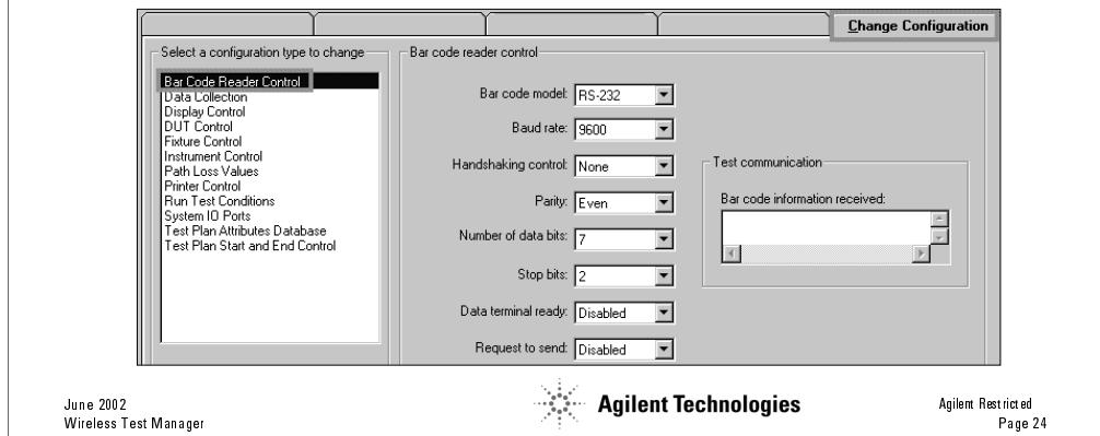
Use the Test communication box to test the communication between your bar code reader and the Wireless Test Manager.
