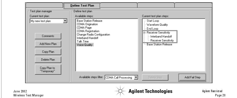
A fail step is run only if the step that it is added to fails. Specifications and parameters for a fail step are set independently of other steps in a test plan.
