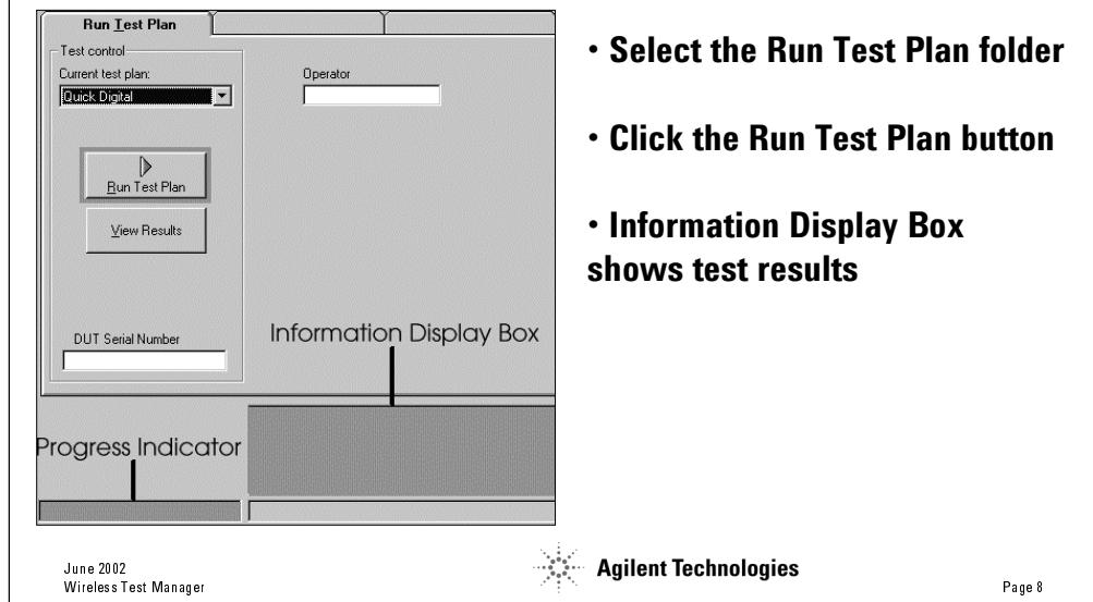
Running a test plan is the most common task you are likely to want to perform with the Wireless Test Manager.
