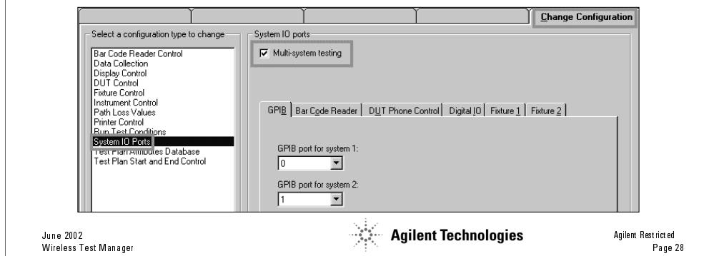
The Wireless Test Manager supports testing on one or two test systems.
