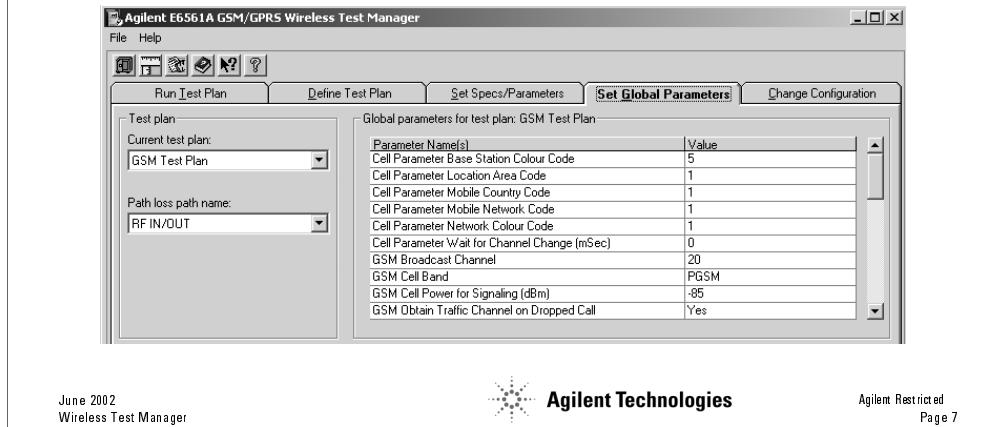
A global parameter is different from a parameter which is assigned to a specific step. A step parameter only affects the individual step to which it is assigned, whereas a global parameter affects all steps within a test plan.
